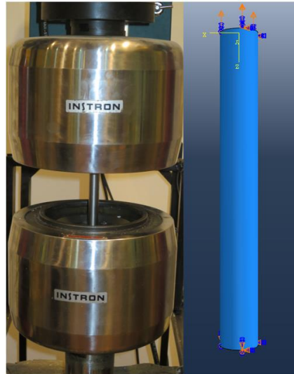
Figure 4 - Photo of the 15PIN235 pin before the test (left); geometry and boundary conditions of the corresponding numerical model in Abaqus .
